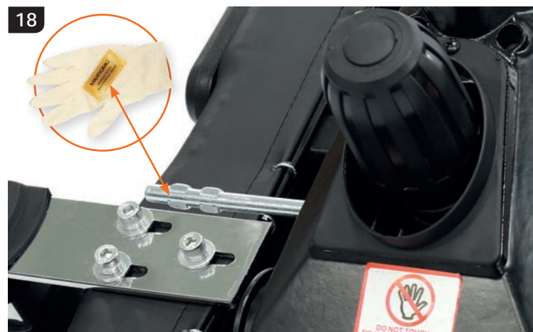
18 Grease the axles of the tilt mechanism lightly. This will make the assembly of the plastic levers easier.
